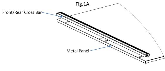
Insert the 3 back positioning screws of Cross Bar into the keyhole slots and then slide into locking position
