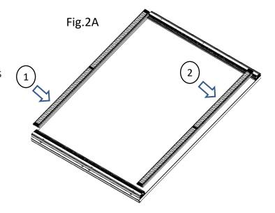
Press Individual Roller Tracks into Cross Bar until snapped into place
